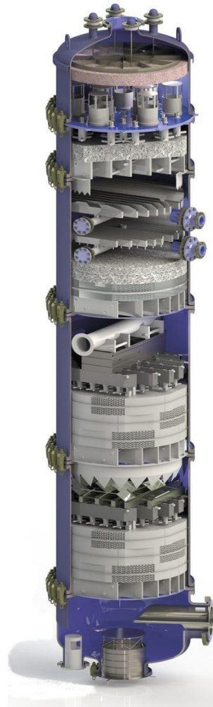
Figure 4. DeDietrich focuses on columns and internals for highly corrosive processes at temperatures up to 390°F. Columns up to DN1000 are made of QVF borosilicate glass 3.3 or DeDietrich glass-lined steel. Bigger columns up to DN2400 are made of DeDietrich glass-lined steel only.
